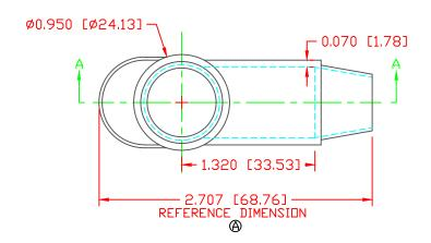
ALL DIMENSIONS GIVEN AS: in [mm] MOLDED PARTS: ±.030" [±0.8mm] HARDWARE ITEMS: ±.010" [±0.25mm]
